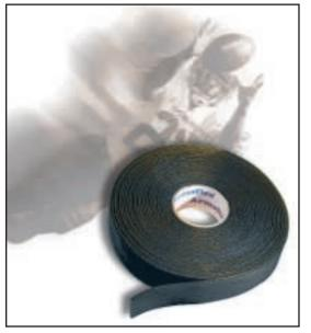
adhesive adheres firmly and forms a long-lasting bond with metal surfaces. On cold piping, the number of wraps required must be sufficient to keep the outer insulation surface above the dew point of the air so that sweating will be controlled. On hot lines, the number of wraps is dictated only by the amount of heat loss control that is desired. On dual-temperature lines, any number of wraps sufficient to control sweating on the cold cycle is usually adequate for the heating cycle.
